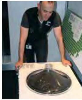
Pellets bounce to the rhythm of the speaker membrane, varying in pattern as the frequency is changed
