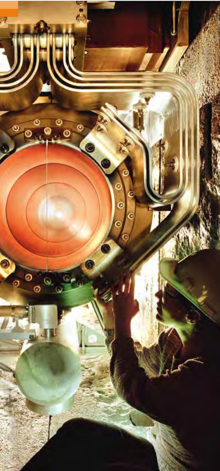
Fermilab is America's leading particle physics laboratory and operates the world's most advanced particle accelerators. Scientists use particle accelerators to research some of the least understood particles in the universe: neutrinos. A vibration analysis project recently helped discover the cause of a small fracture in the powerful magnetic horn used to send neutrino beams to Minnesota.
