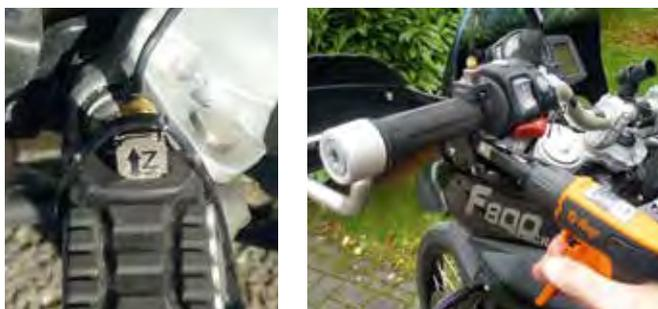
To ensure the reproducibility of the measurements, the accelerometers were mounted with cable straps and a tool to tighten the straps with always the same force
