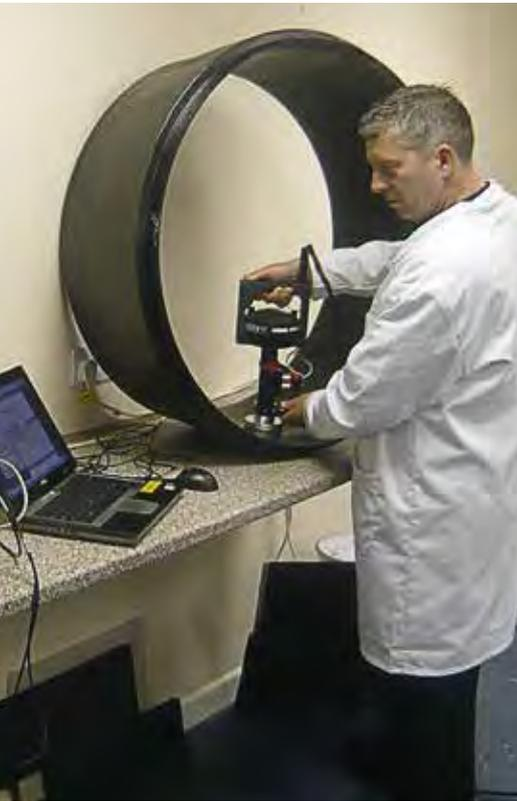
Impedance testing of a GKN Aerospace zero splice acoustic panel
