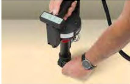
Portable Impedance Meter Type 9737 is a user-friendly kit for quick, non-destructive acoustic material testing
