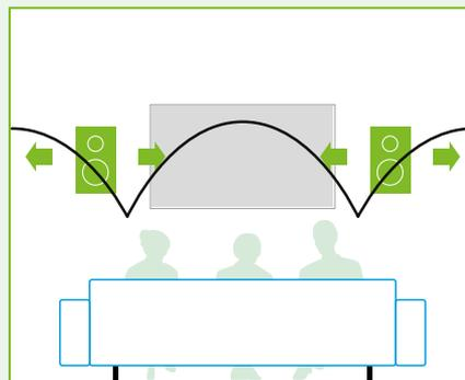
Match for the next higher frequency, where two wavelengths fit into the room: Strong sound at the walls and again in the middle of the room, alternating with areas of weak sound
