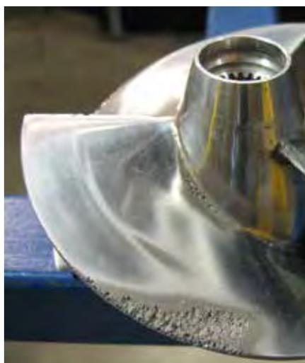
Along with noise, when a steam bubble implodes, it creates a micro-jet that, over time, can result in considerable damage to materials in the immediate vicinity
