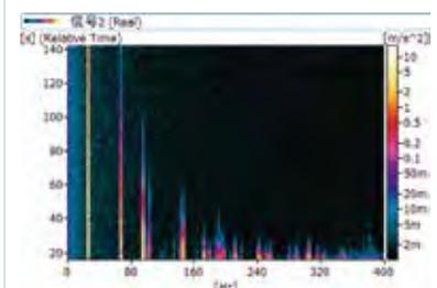
The vibration signal takes more than 140 seconds before decaying, shown by the FFT vs time and total slice, which shows the most prominent tone to be around 26 Hz. Beating frequencies were also found when the bell was vibrating
