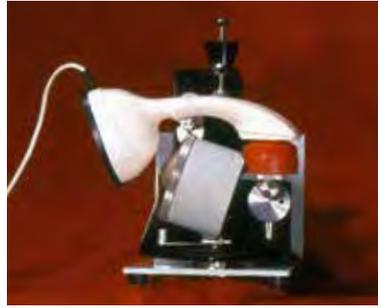
Telephone Test Head Type 4905 – shown testing Ericsson's 'Eriocofon', also known as the cobra telephone (photo ca. 1970)
