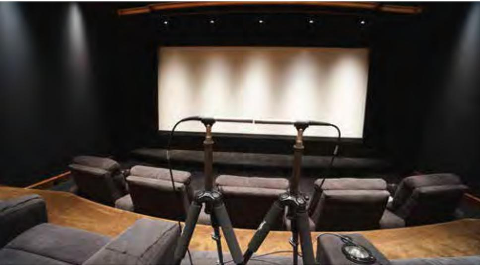
Two-microphone coherent power measurement technique set-up
