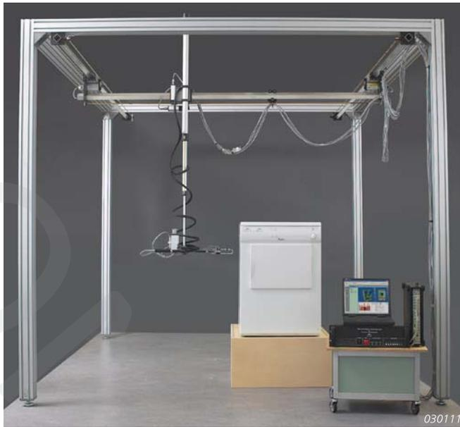
A fully automatic system is normally based on a five-axis robot for single microphones, intensity probes or smaller arrays.
