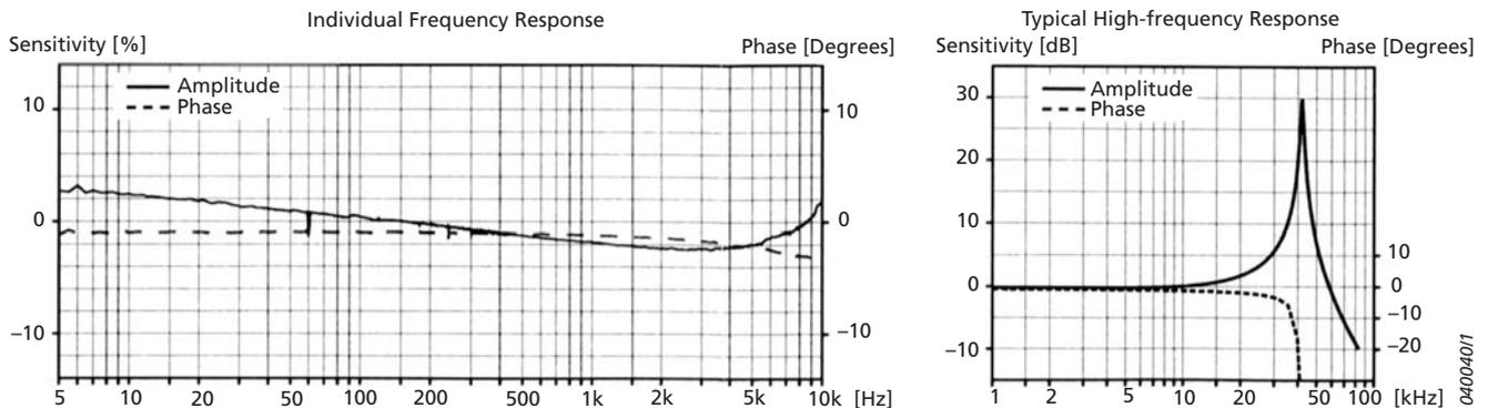
\* Unigain: The individual measured sensitivity is within  $\pm 2\%$  of the specified sensitivity
