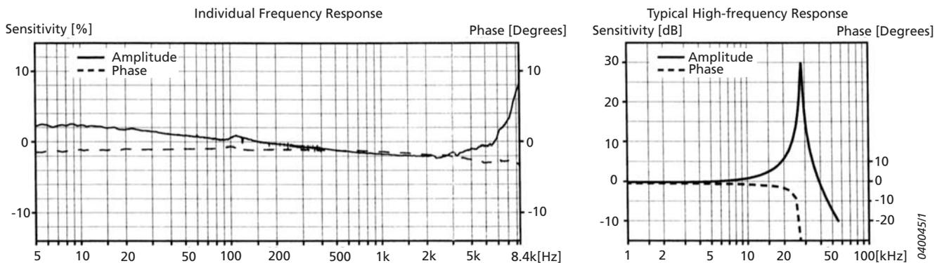
\* Unigain: The individual measured sensitivity is within  $\pm 2\%$  of the specified sensitivity
