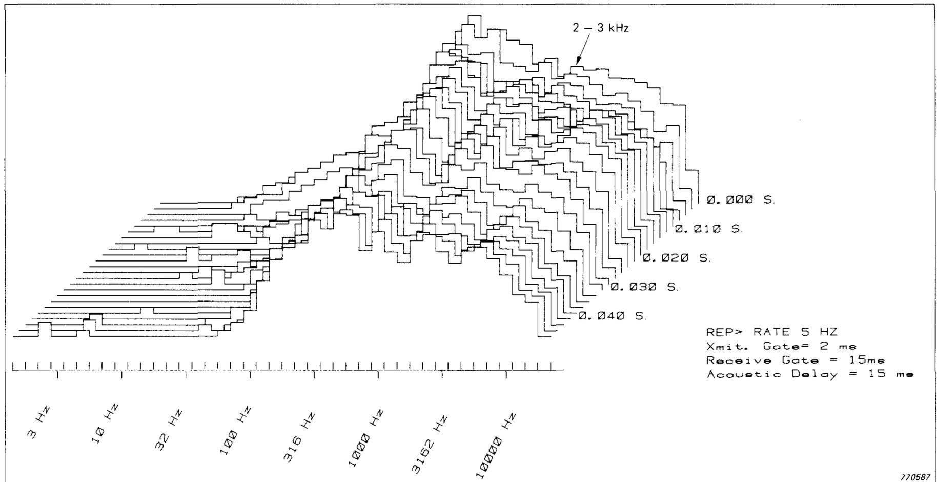
Fig.19. 3 D plot of lecture room showing how the frequency spectra change with time. 0—50 ms time axis. Receiving gate 15 ms
