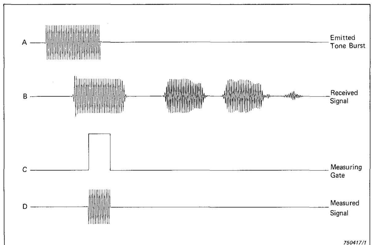
Fig. 1. Principle of gated measurements
