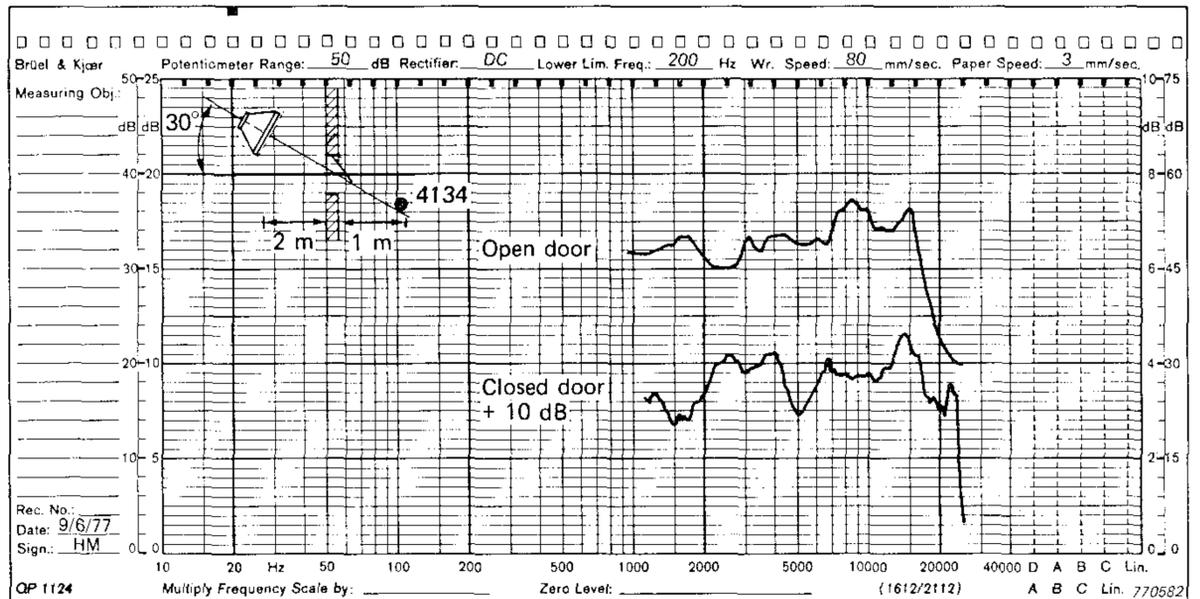
Fig.28. Spectra of conventional door open and closed.  $30^\circ$  off axis
