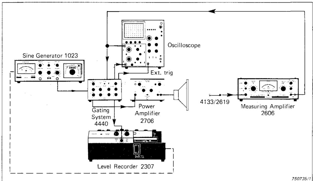
Fig.3. Set-up using Gating System
