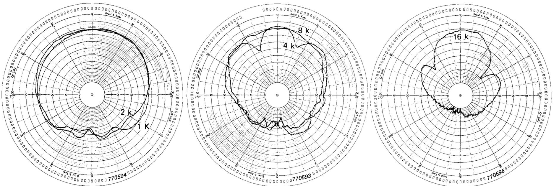
Fig. 9. Directional characteristics of the loudspeaker used
