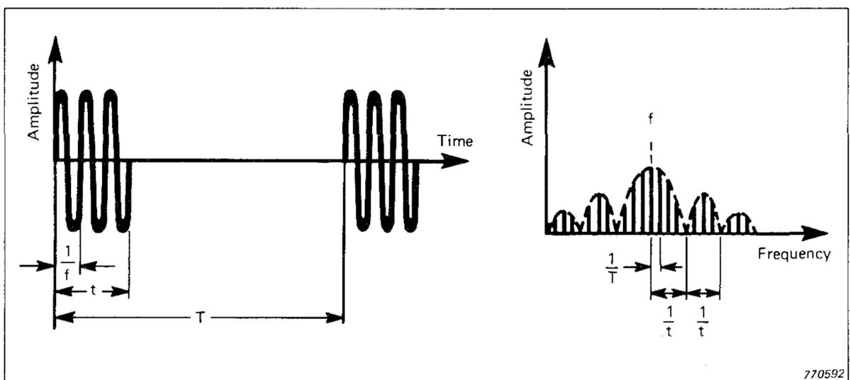
Fig.4. Time and frequency spectra of gated sine wave. Notice that a narrow time spectrum corresponds to a broad frequency spectrum and vice versa
