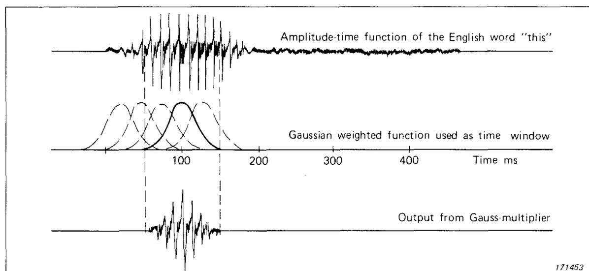
Fig.27. The operation of the Gauss Impulse Multiplier 5623
