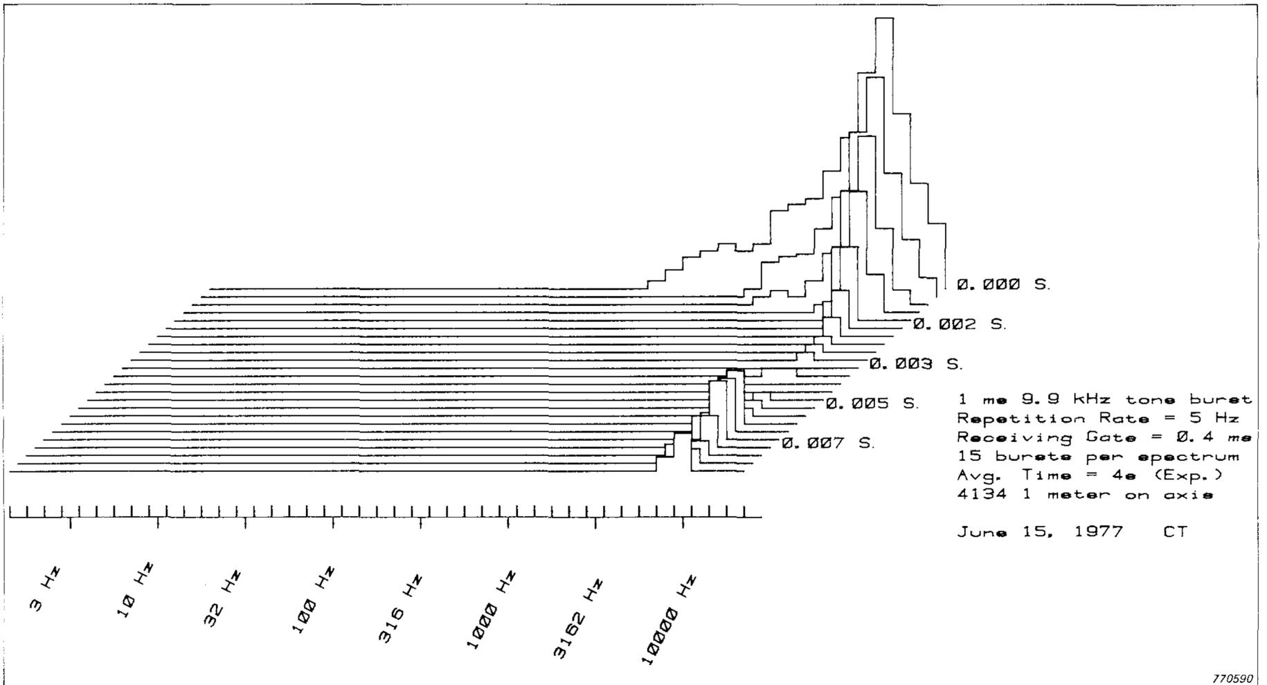
Fig.20. 3 D plot of Early Reflection of loudspeaker. Time 0—8 ms. 1 ms 9,9 kHz tone burst
