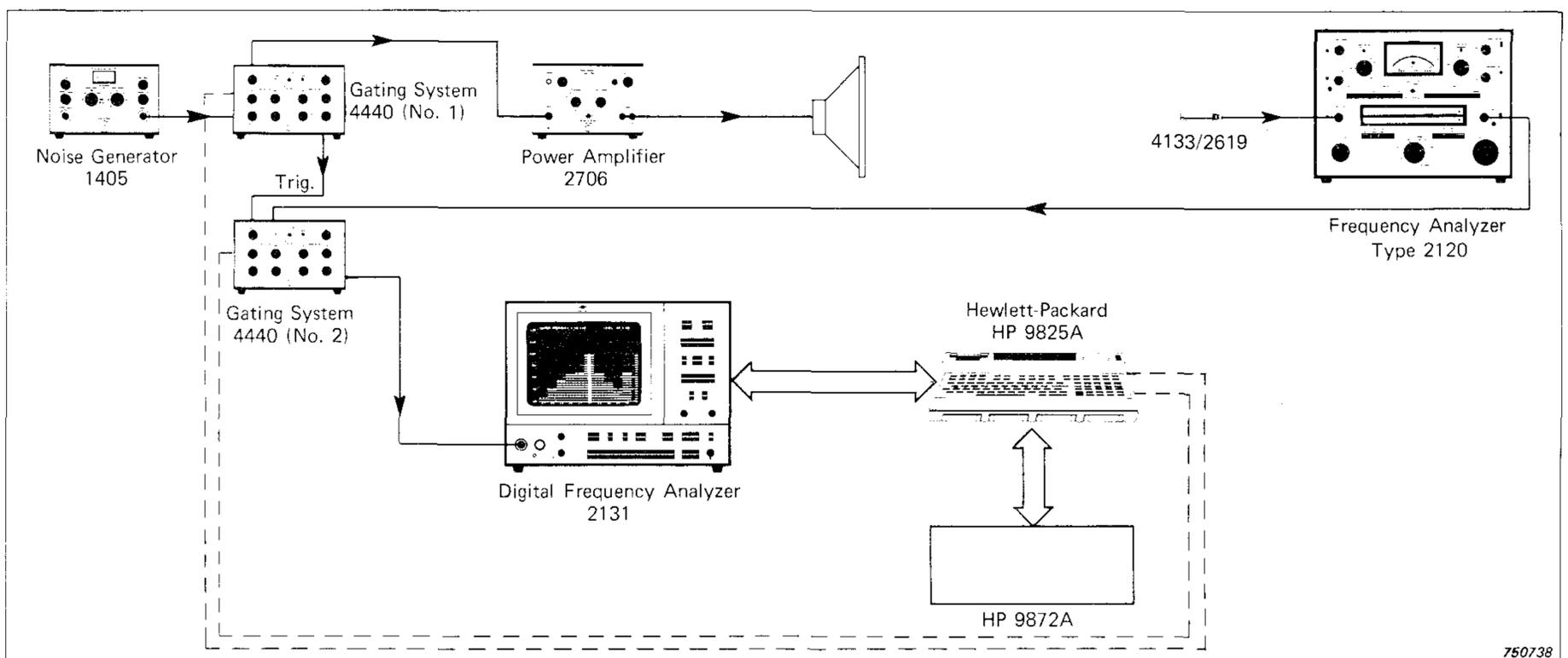
Fig.15. The instrument set-up using gated pink noise, real-time analysis and automatic control by calculators
