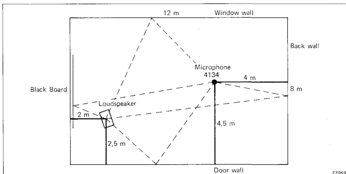
Fig.7. Schematic drawing of the lecture room
