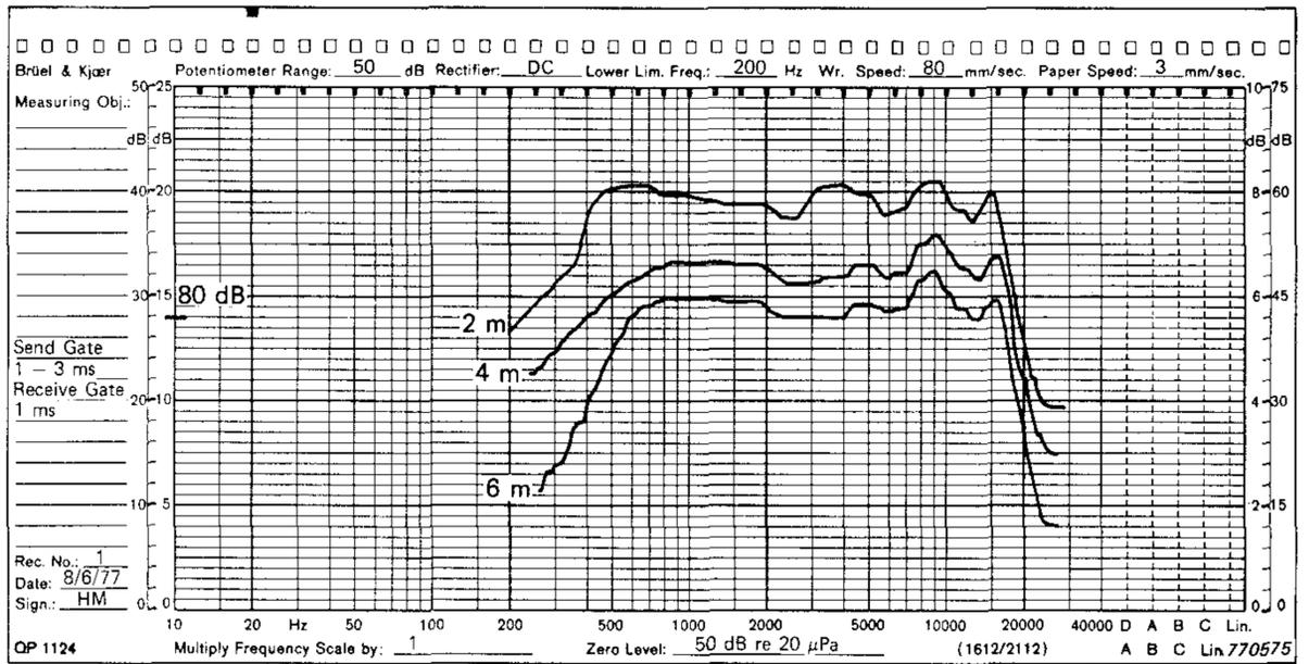
Fig. 8. "Free-field" measurements of the loudspeaker used
