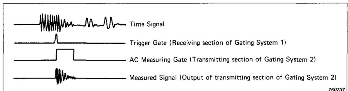
Fig.29. Setting of gates to measure early reflections with the instruments in Fig.28
