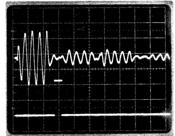
Fig.26. Adjustment of the gate for measurement of early reflections
