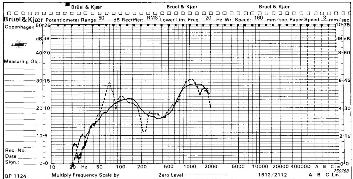
Fig.18. Illustration of averaging due to too short a tone burst. Dashed line shows free-field sine wave response, solid line shows the response measured with a tone burst consisting only of one period of its frequency
