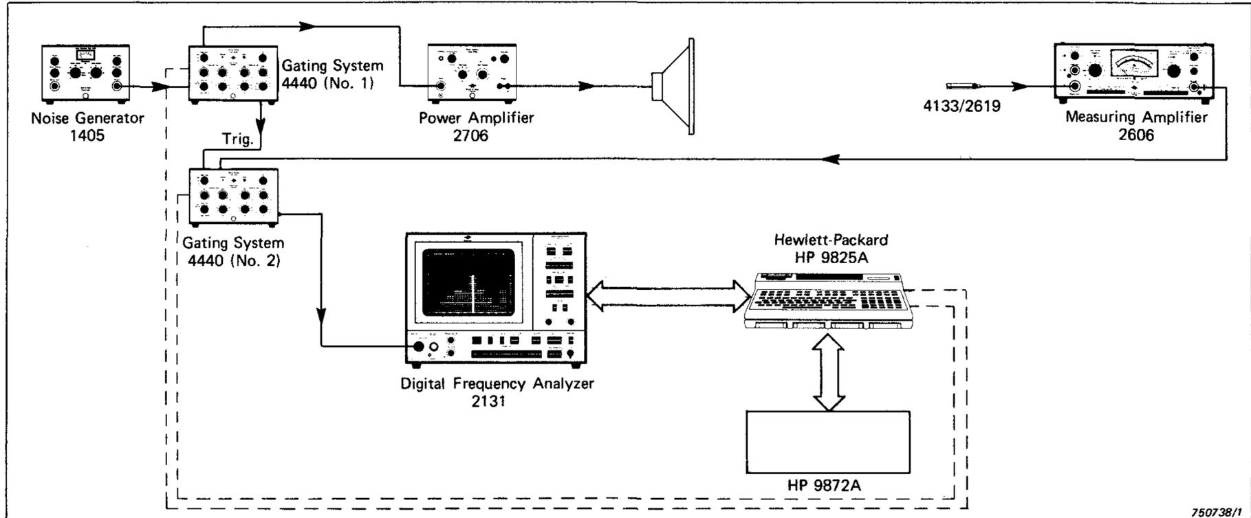
Fig.28. Instrument set-up for real-time analysis of early reflections using gated white noise
