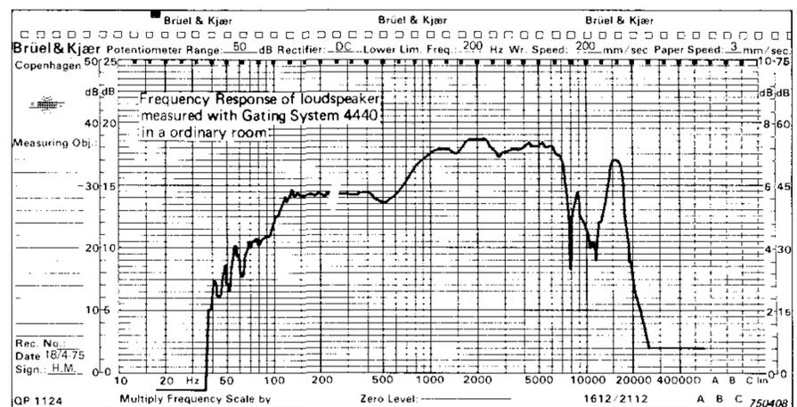
Fig.9. Frequency response of the same loudspeaker measured with the Gating System in an ordinary room
