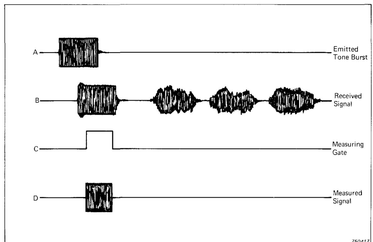
Fig.1. Principle of the Gating System
