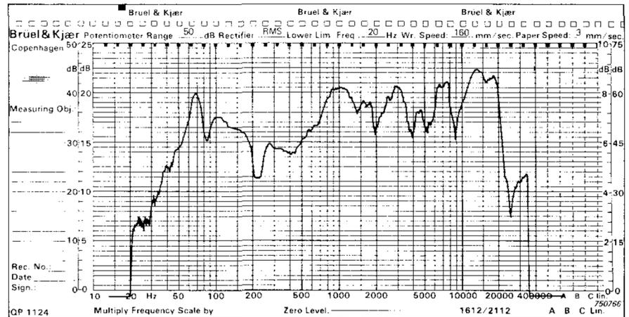
Fig.11. Frequency response of a loudspeaker (not the same as in Figs.8 and 9) using pure sine in anechoic room
