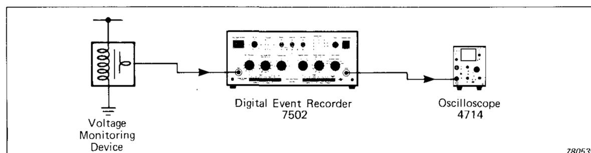
Arrangement of equipment for capturing and measuring line voltage surges
