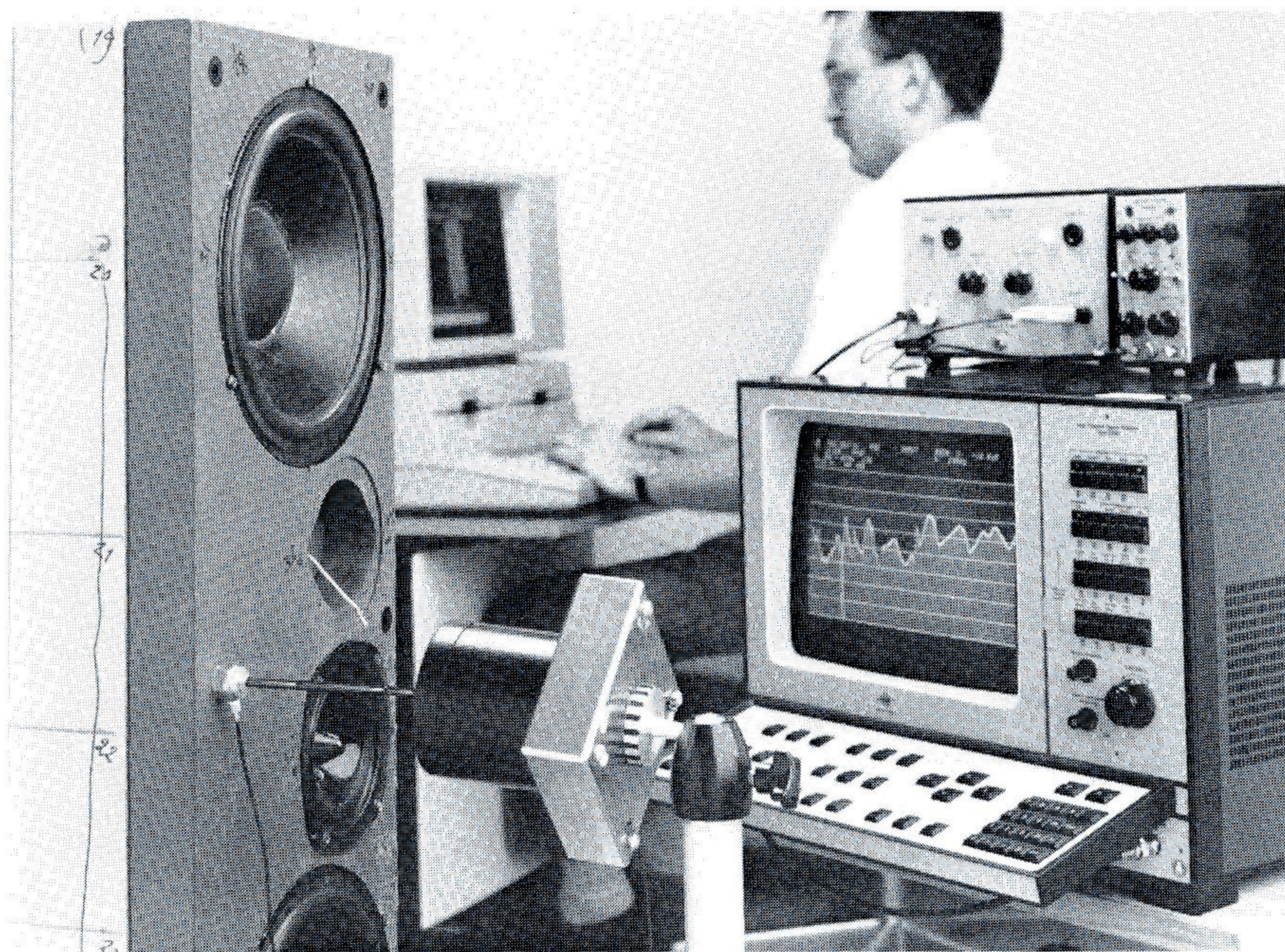
Modal analysis of a hi-fi loudspeaker. The Dual-Channel Signal Analyzer Type 2032/2034 is used to measure the compliance between the driving point and a number of response points; then a computer aids the extraction of the mode shapes.
