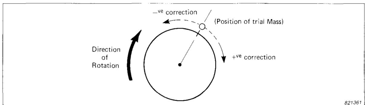
Fig. 9. Determining the position of the correction mass
