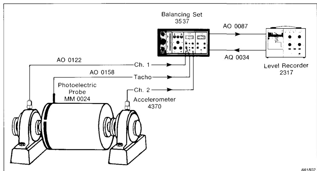
Fig. 26. Two-plane balancing with the Type 3537 Balancing Set
