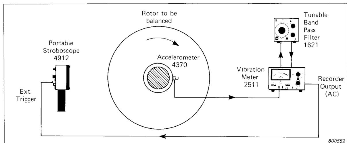
Fig. 27. Using a stroboscope to measure phase angles
