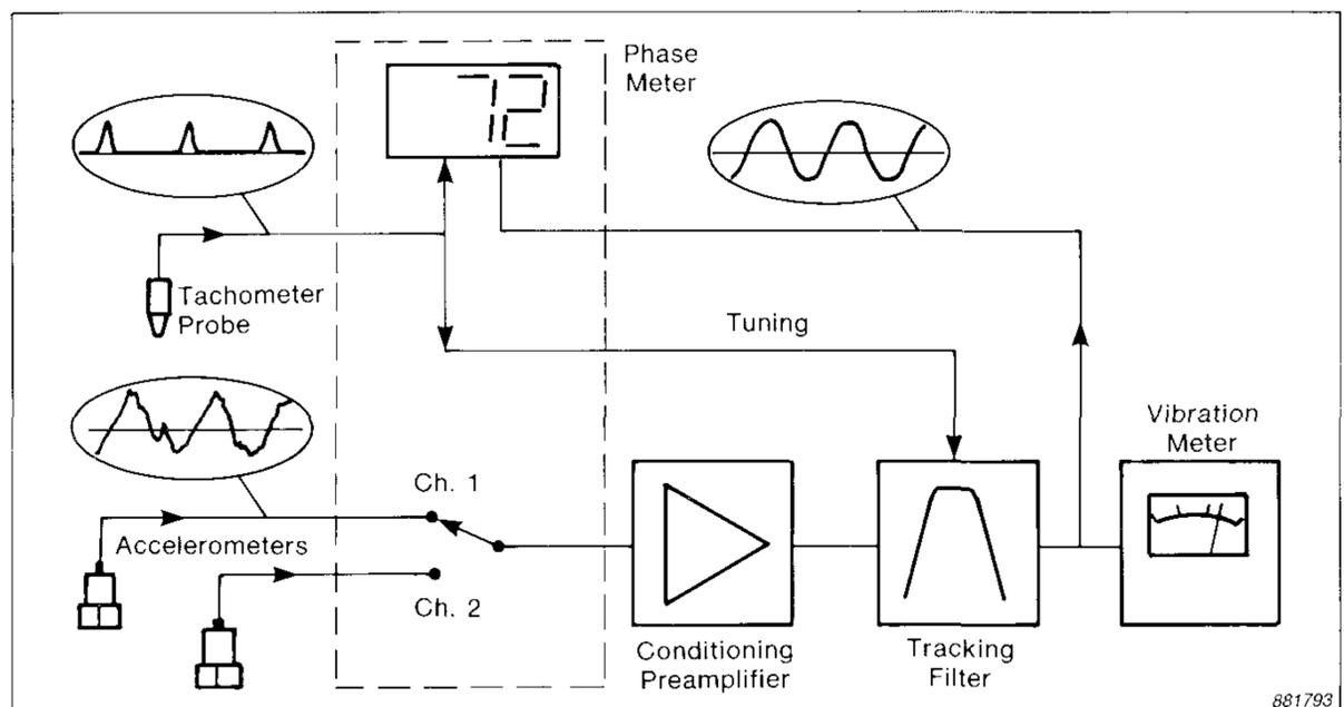
Fig. 25. Signal paths in the Type 3537 Balancing Set
