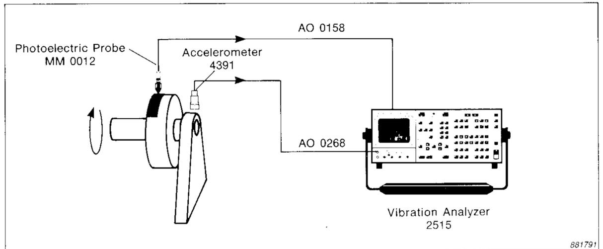
Fig. 20. Single-plane balancing with the Type 2515 Vibration Analyzer
