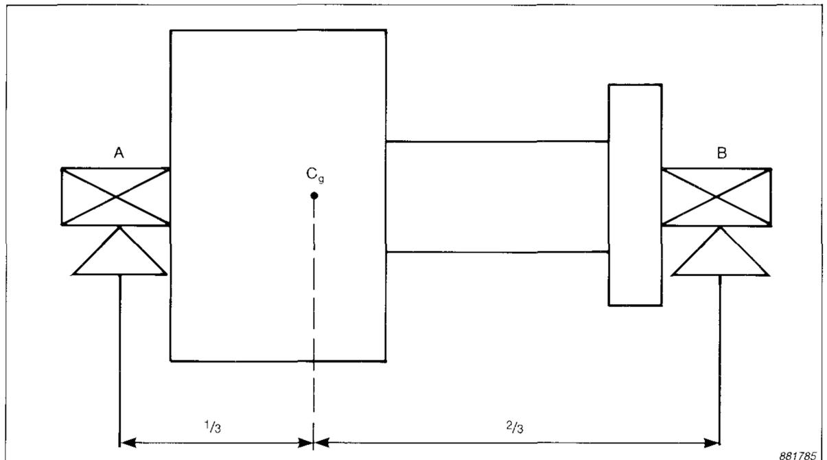
Fig. 8. A rotor with unevenly distributed mass
