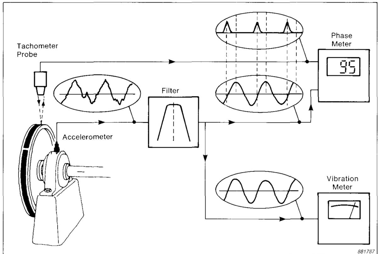
Fig. 5. The basic measurement chain
