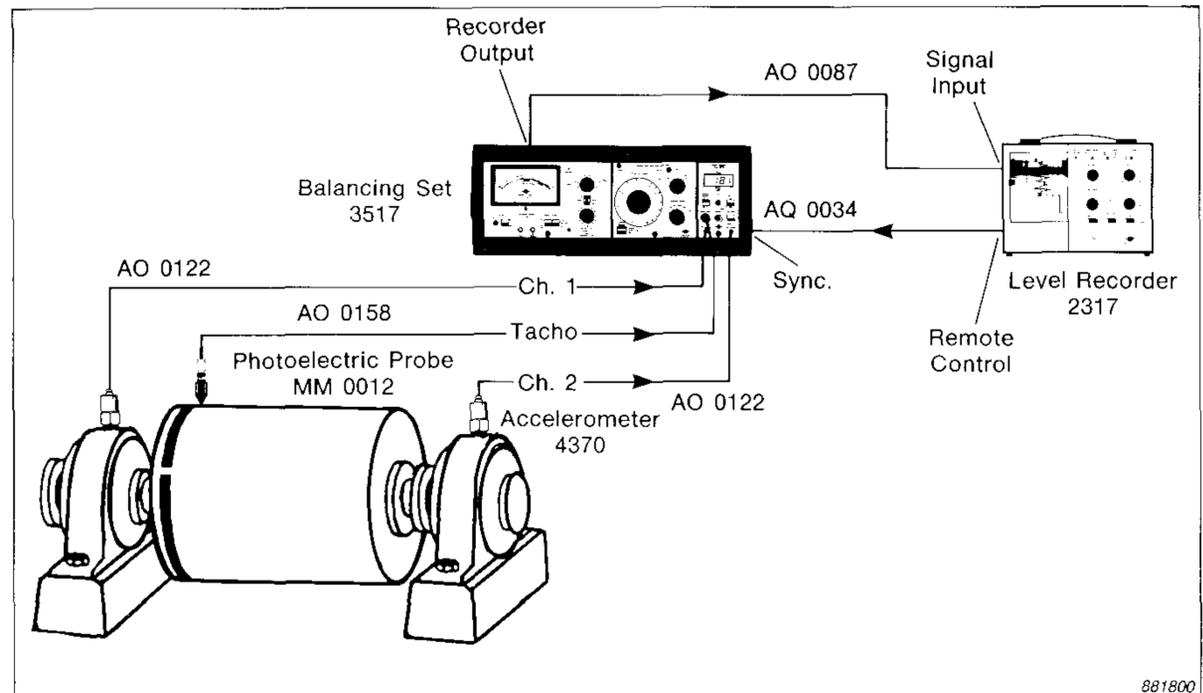
Fig. 23. Two-plane balancing with the Type 3517 Balancing Set
