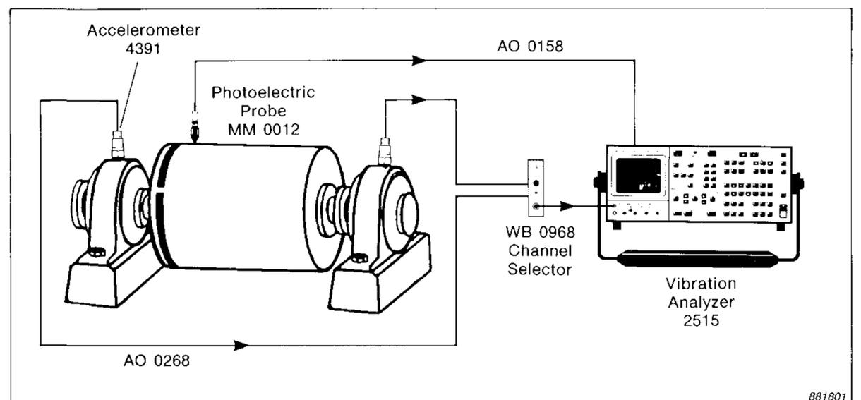
Fig. 31. Instrument set-up for Example Two
