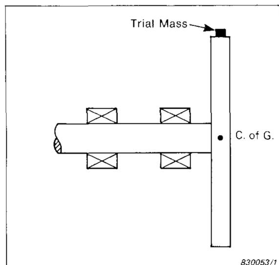
Fig. 11. Overhung rotor balanced using a single-plane procedure
