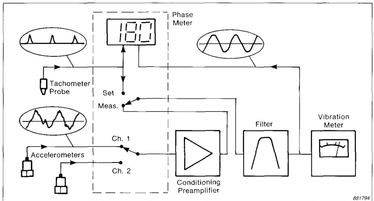
Fig. 22. Signal paths in the Type 3517 Balancing Set
