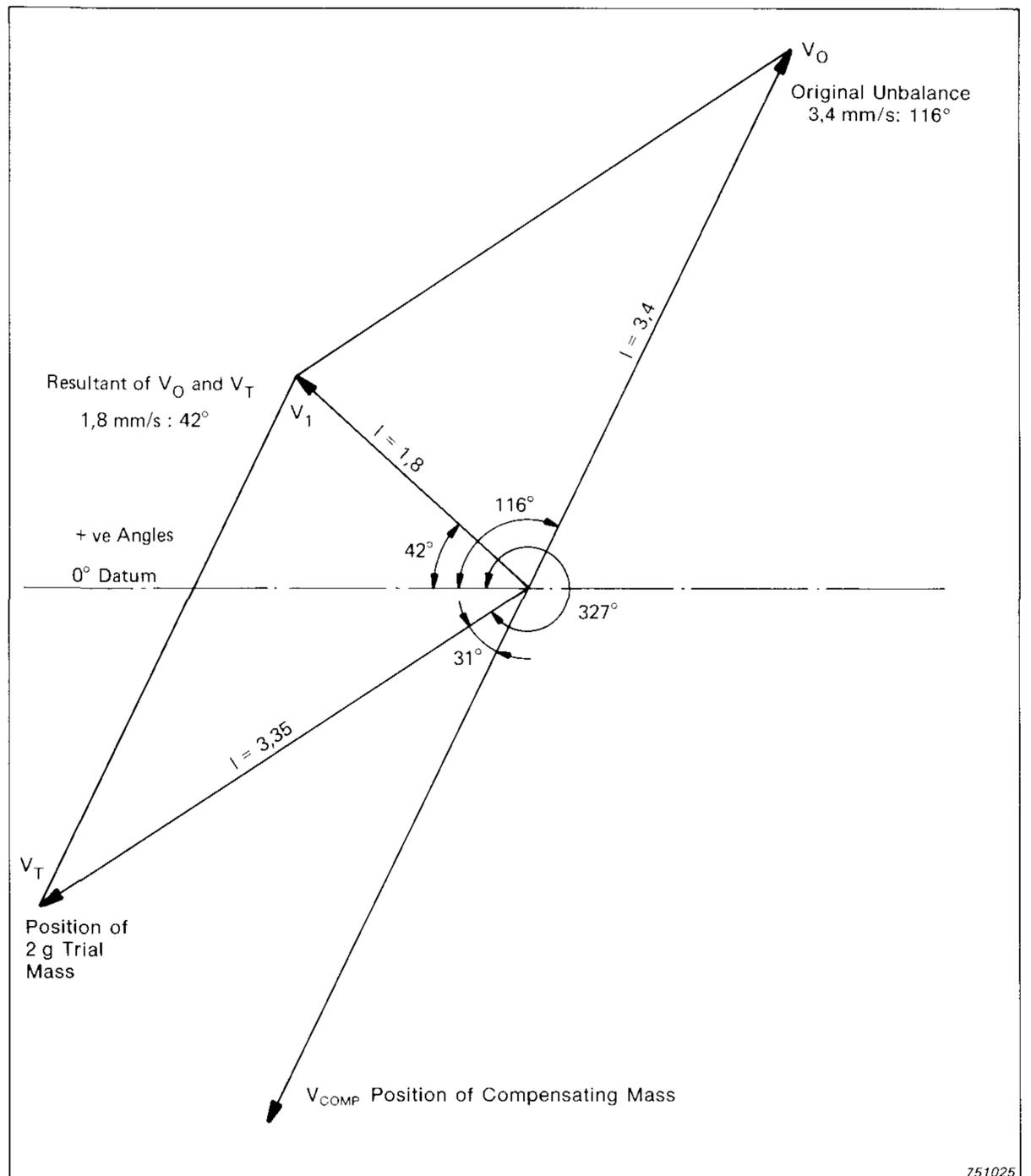
Fig. 30. Vector diagram for Example One
