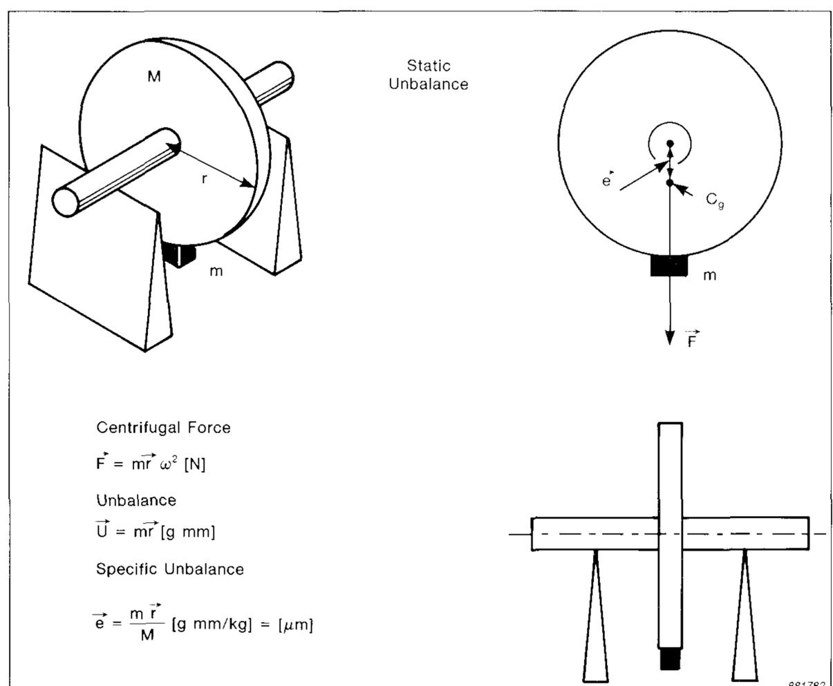
Fig. 1. Static unbalance
