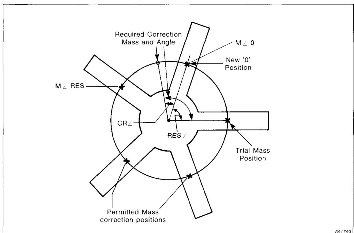
Fig. 18. Dividing a correction mass into two components for mounting on a five-blade fan
