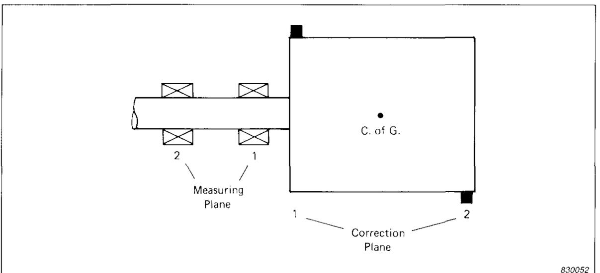
Fig. 13. Overhung rotor balanced using a two-plane procedure
