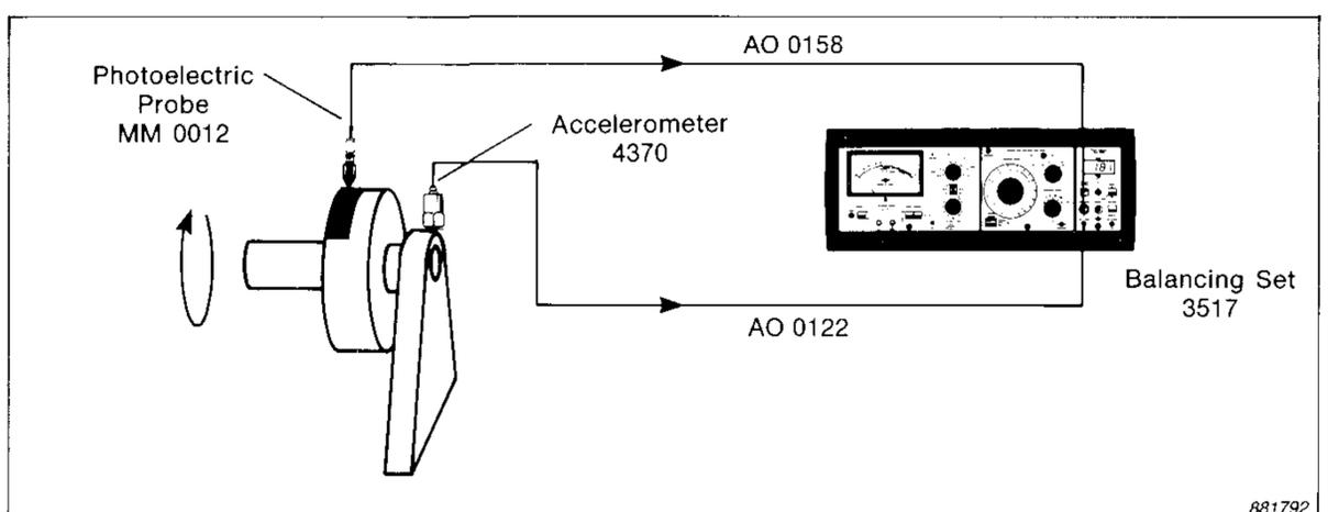
Fig. 29. Instrument set-up for Example One
