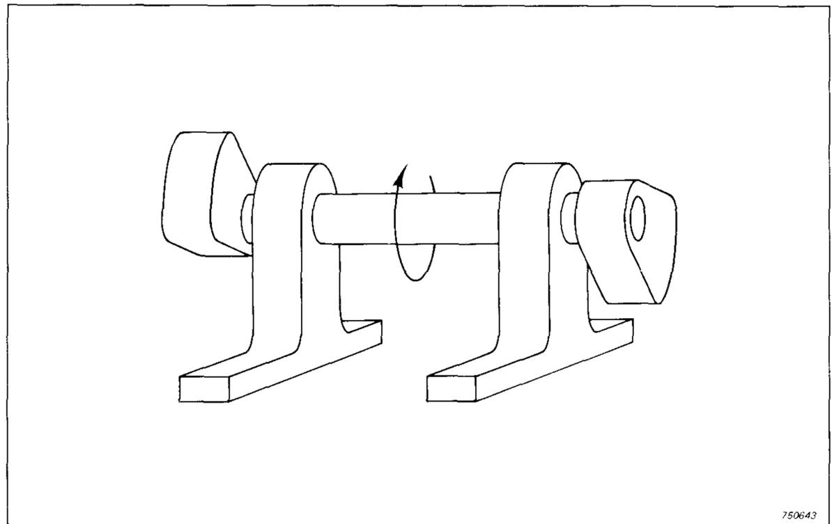
Fig. 3. Static balance, couple unbalance
