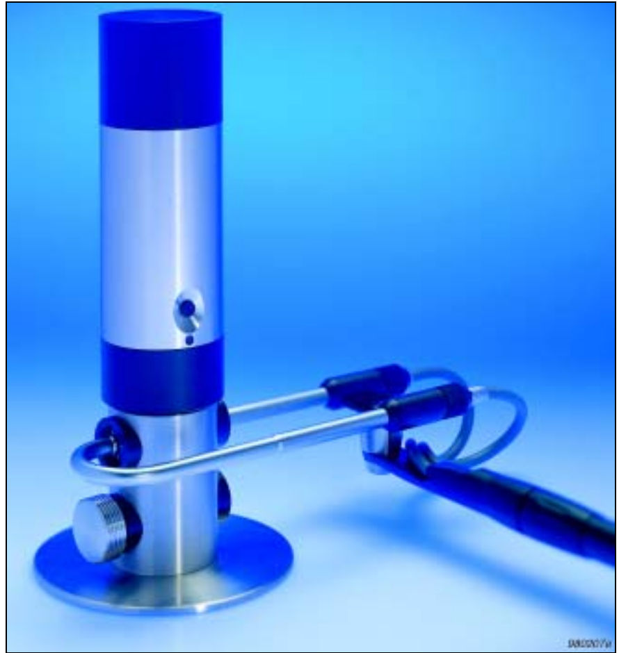
Fig. 12 Complete calibration of sound intensity measurement systems containing a sound intensity probe set can be conveniently made using a Sound Intensity Calibrator Type 3541. This permits simultaneous sensitivity adjustment of both channels of the processor (in both pressure, particle velocity or intensity modes) and allows determination of the Pressure-Residual Intensity Index of the probe and processor combinations which employ microphone pairs with phase-corrector units, i.e., Type 4197. Further details can be found in the separate Product Data for Type 3541
