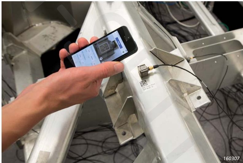
Fig. 2 Using the Transducer Smart Setup app to scan the data matrix code on the transducer and the label next to the transducer ensures fast and correct DOF information for the measurement
