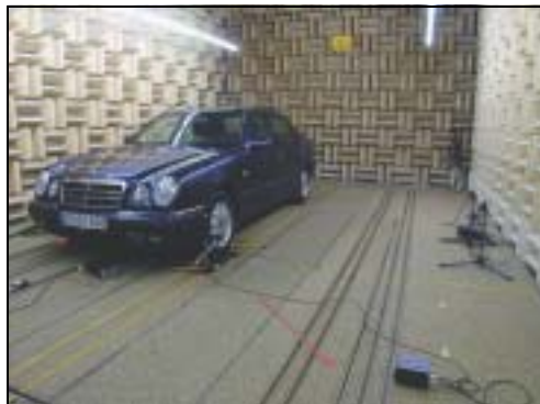
Fig. 2 The semi-anechoic test cell at Pirelli's Höchst facility
