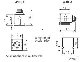
Types 4500-A, 4501-A and 4501-A-001 are piezoelectric charge accelerometers with ThetaShear design.
