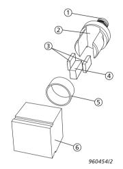
Types 4500-A, 4501-A and 4501-A-001 have high measurement stability and excellent sensitivity-to-weight ratio due to the ThetaShear design. In addition, the transverse resonance frequency is always outside the 10% frequency limit. This ensures minimum interference from orthogonal vibration components in the useful frequency range of the accelerometer. The ThetaShear design also provides excellent immunity to environmental effects such as base strains, magnetic sensitivity and acoustic fields.
