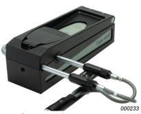
Phase calibration of ½" Microphone Pair Type 4197 is done at HBK by subjecting the two microphones to the same sound signal in a pressure coupler. This individual phase calibration can be used to derive the actual Pressure-Residual Intensity Index for the microphone pair.
