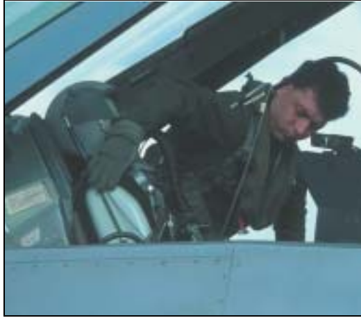
Fig. 3 Captain Casper B. Nielsen of the Danish Tactical Air Command checks that the HATS harness is securely fastened
