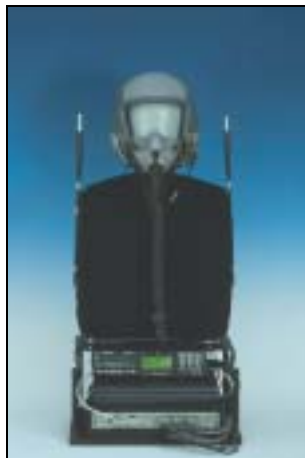
Fig. 2 The test setup comprising HATS, PULSE Multi- analyzer and SONY® DAT recorder
