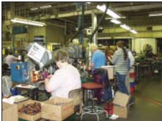
Fig. 3 The assembly lines at Motor Products are highly manual – the wide product range and variable order quantities suits this type of operation
