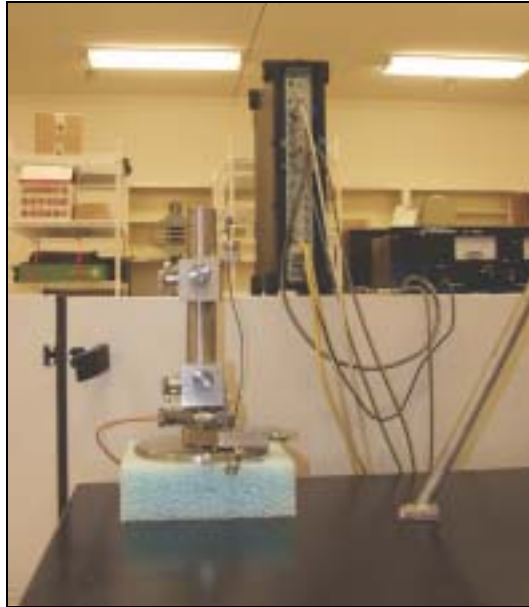
Fig. 5 A 4-channel PULSE system was purchased four years ago. The Complex Modulus Apparatus is used to test the vibration damping characteristics of materials
