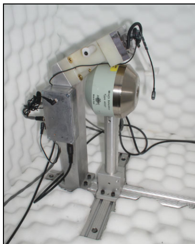
Fig. 6 Inside a small anechoic chamber in the R&D lab, a Brüel & Kjær Mouth Simulator Type 4227 is connected to SoundCheck™, via an amplifier. This setup is used to test the response of the microphone Photo by kind permission of Shure Incorporated
