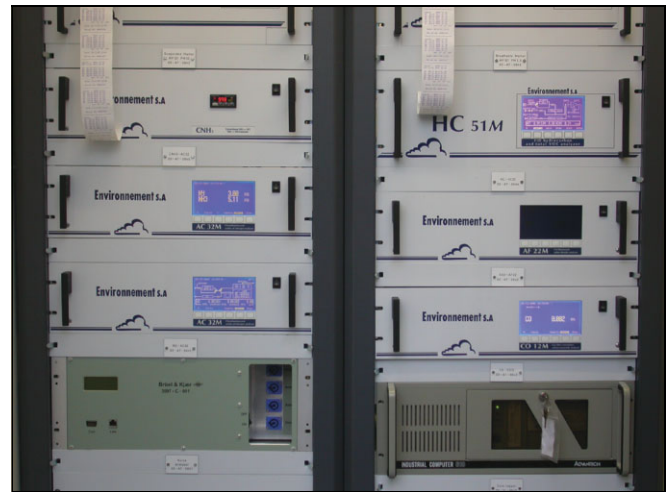
Fig. 1 Example of the finalised Oman India Fertilizer Company turnkey system Left: Permanent monitoring station; Right: Close-up of rack setup within station containing various Environnement S.A. analyzers and Brüel & Kjær's noise level analyzer
