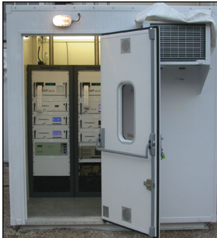
Fig. 1 Example of the finalised Oman India Fertilizer Company turnkey system Left: Permanent monitoring station; Right: Close-up of rack setup within station containing various Environnement S.A. analyzers and Brüel & Kjær's noise level analyzer
