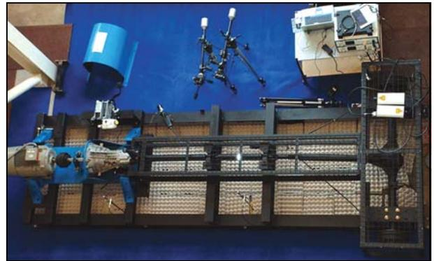
Dr. Gnanakumarr explains, "A metallic noise is often heard when rapidly engaging and releasing the clutch. This is known in industry as 'clonk'. It is especially prevalent on vehicles with rear wheel-drive. The driveline shafts are hollow steel tubes and these tend to act as loudspeakers and amplify this metallic noise".
