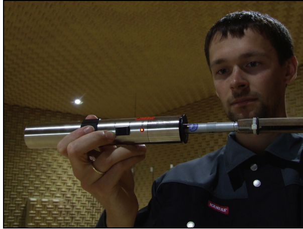
Fig. 1 An engineer performing the weekly pistonphone calibration
