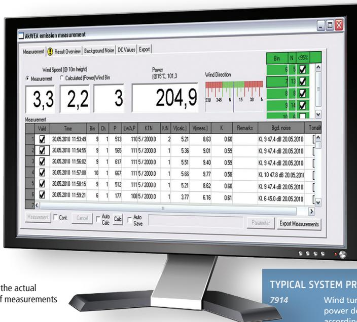
Typical measurement with the actual indication of the number of measurements per wind bin.
