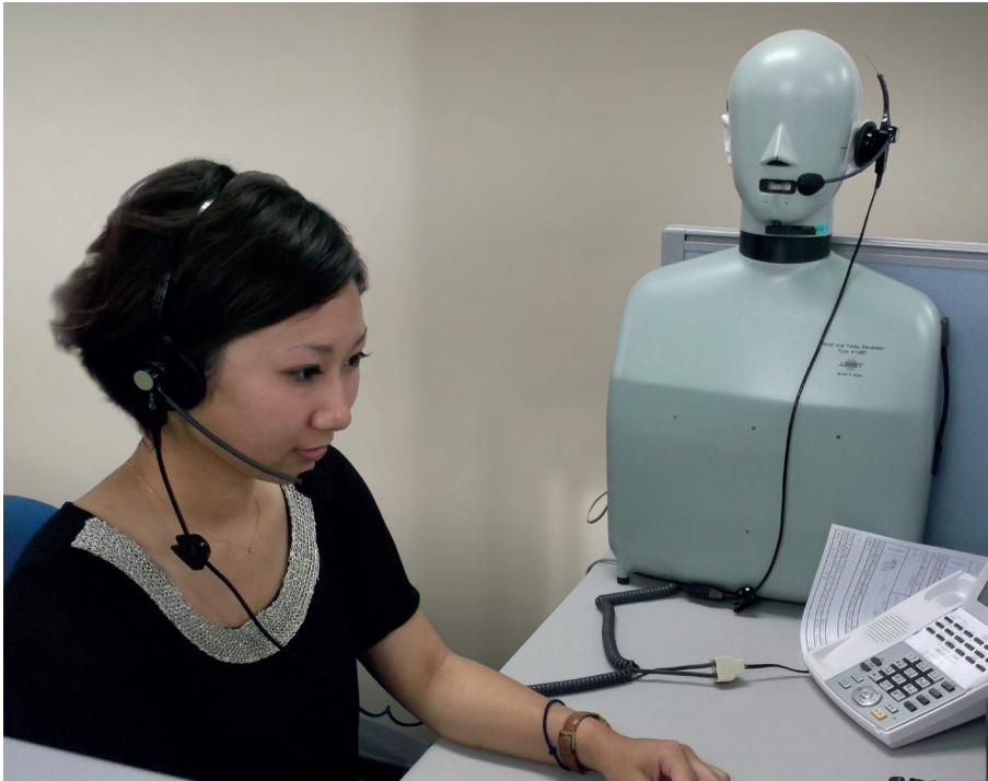
The HATS was used in parallel with workers making real calls, so the incoming call signal from the telephone was divided between two headsets
