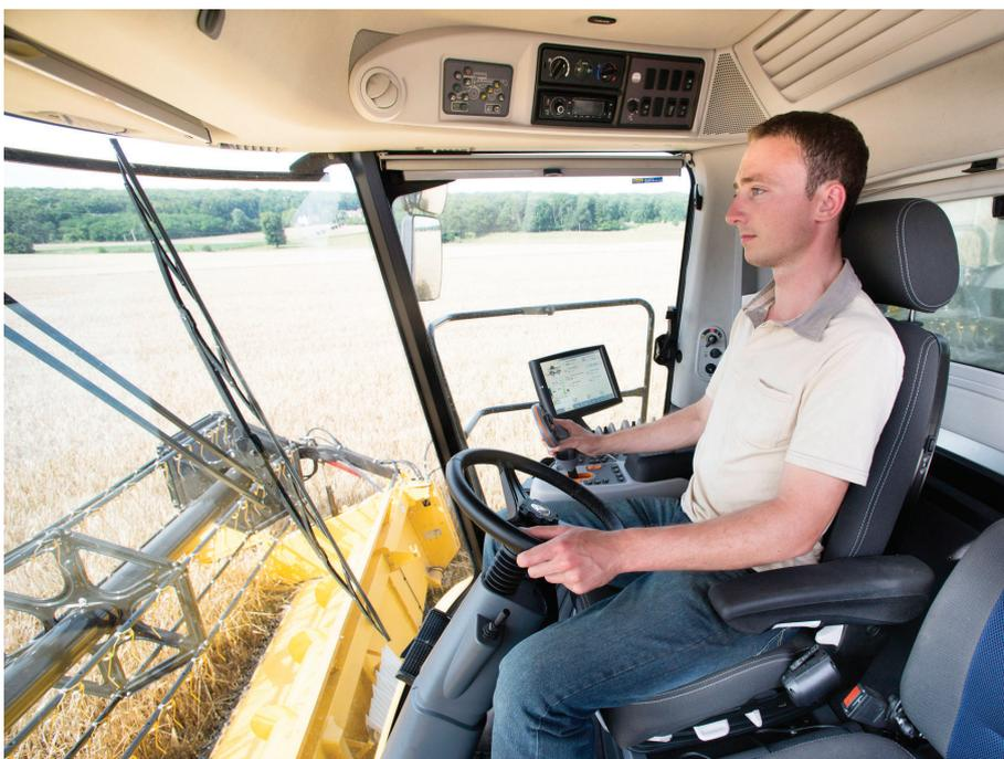
*Comfort reduces the driver's fatigue, and New Holland's Harvest Suite cab leads the market with a 73 dB(A) noise level thanks to significant investigations into glass layups combined with frequency-optimized materials*
