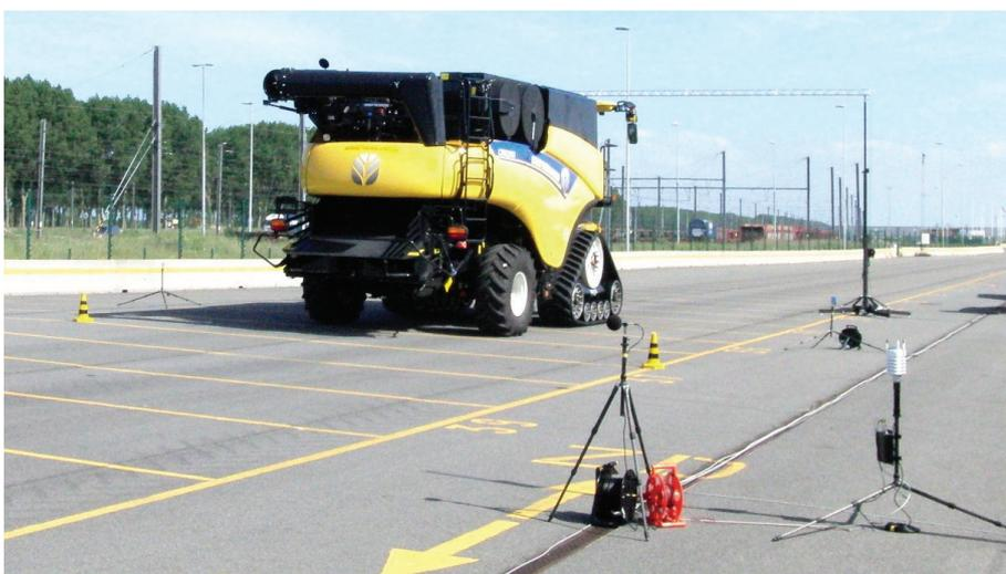
*Without any suspension, combines present challenges for pass-by testing. The standard dictates a sudden full-throttle acceleration, which makes the machines rock back and forth, causing noise oscillations*
