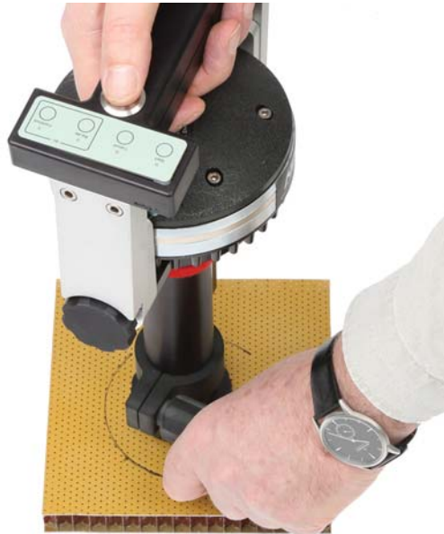
Fig. 2 Type 9737 being used on an acoustic panel sample
