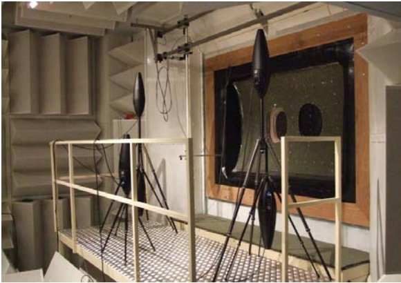
Fig. 8. Set-up with 5 speakers in Transmission Loss facility at Dassault Aviation, France. View from anechoic room.
