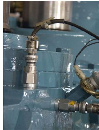
7b. Magnet mounting of the roving transducers
