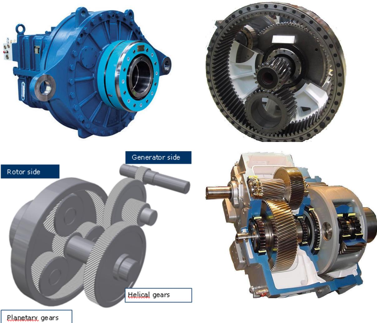
Figure 6: Gearbox and examples of gears from Wind Turbines
