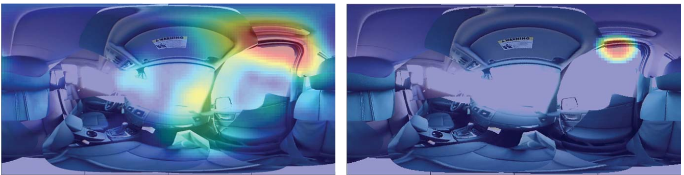
Fig. 8 Spherical beamforming used to investigate noise in the gangway of a high-speed train. The map shows the 1600 Hz third-octave band
