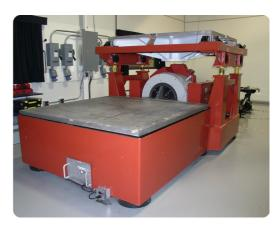
The shaker, used in conjunction with the 8-channel laser controller, is used every day for pre-testing prototypes and package testing. The table can create DOF (X, Y, Z) vibration and products undergo tests in and out of transport boxes and include:
