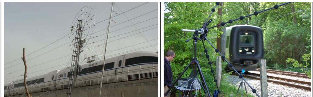
Fig.11. Testing of components on full-sized trains under normal operating conditions: On left, wheel array measuring on high speed train. On right, pentangular array measuring on commuter train
