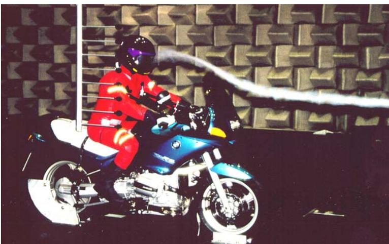
*Fig.2. Near-field holography measurement performed using a robot controlled scan of an array of 8 microphones. A reference microphone is positioned at the motorcyclist's ear to map the sound field coherent with this reference*
