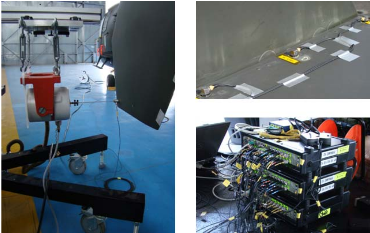
Fig. 3 Examples of test setups Shaker excitation (left), accelerometer mounting (top right) and front-ends (bottom right)
