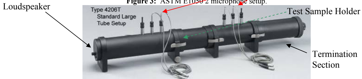
Figure 4: ASTM E2611 4 microphone setup.
