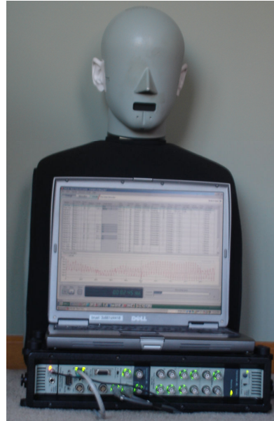
Figure 2. Example of typical measurement equipment: Brüel & Kjær Type 4100 HATS along with Type 3560C PUSLE Hardware front end and Type 7708 Time Data Recorder software
