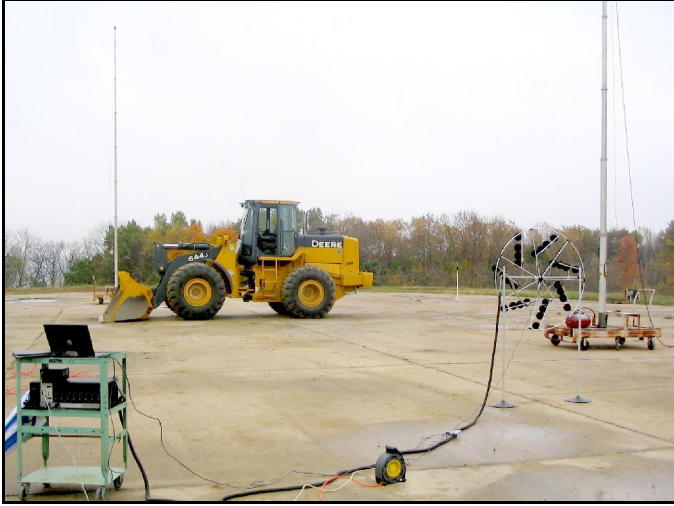
Figure 1. At ground level, the beamforming array was located 15 m from the machine on the sound pad. The two hemisphere microphones located on pneumatic towers can be seen in the background.
