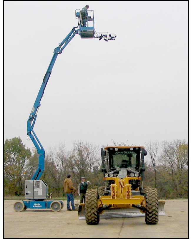
Figure 2. A man lift was used to suspend the array above the machines for the top view.
