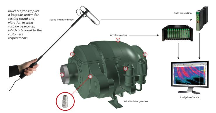
Complete test stands are configured to cover a wide range of components and parameters – down to smaller parts and systems such as brakes, pitch control, yaw motors, and non-rotational bearing stress. Noise detection components are key, as noise is responsible for a significant number of the product warranty returns experienced by Burke E. Porter's customers.
