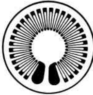
Fig.3.7b. Gauge for measuring radial strain
