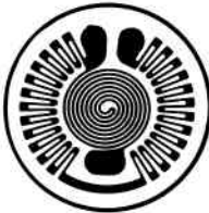
Fig.3.7c. Gauge for measuring radial and/or tangential strain
