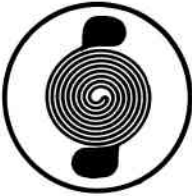
Fig.3.7a. Gauge for measuring tangential strain
