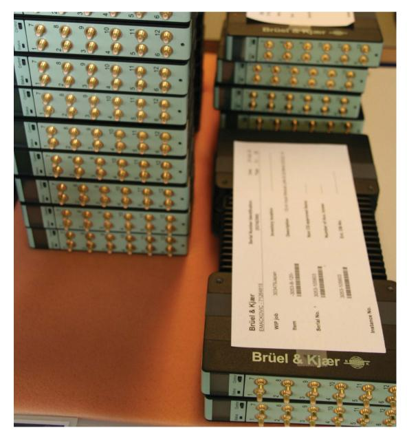
Solutions based on LAN-Xi data acquisition hardware are also expandable to 1000+ channels
