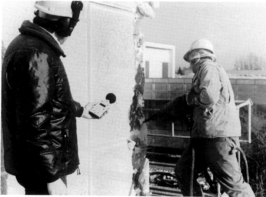
Measuring noise from drilling operations using a hand-held Precision Integrating Sound Level Meter Type 2221 to obtain L_{Aeq,T} and Peak level
