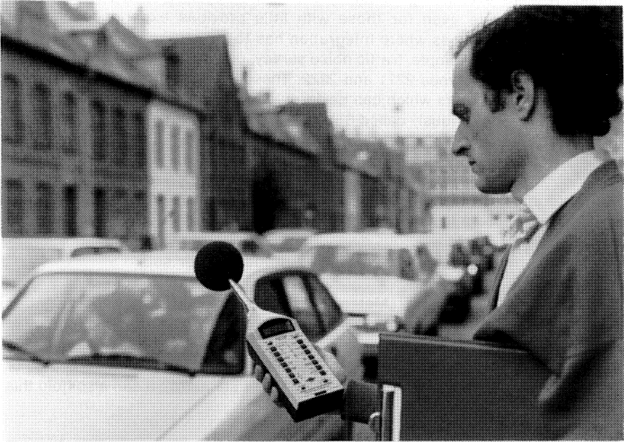
On site traffic noise measurement and statistical analysis with Modular Precision Sound Level Meter Type 2231
