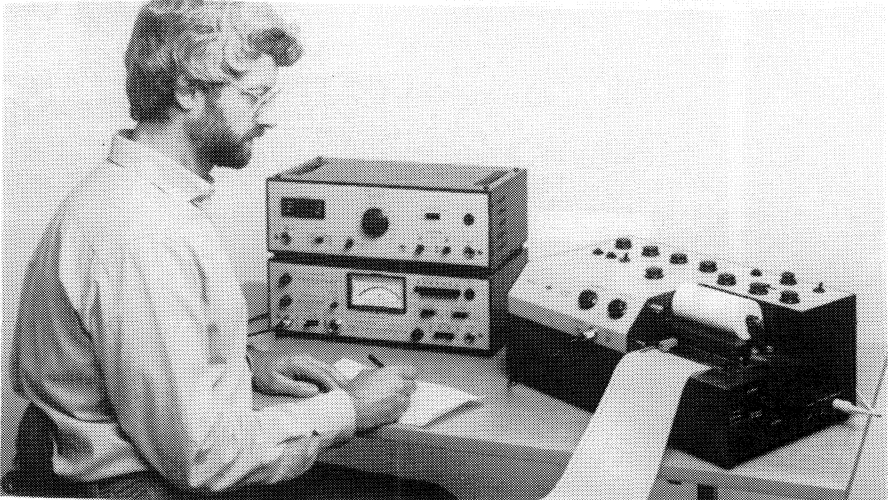
Analysis in octave or third octave bands using a Measuring Amplifier Type 2636 and the Bandpass Filter Type 1617
