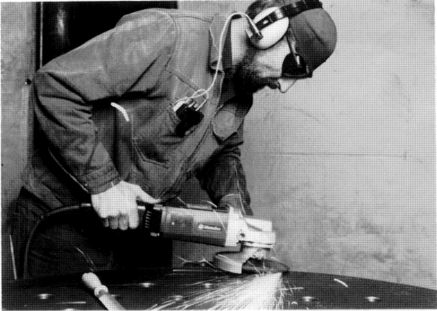
Measurement of noise dose received during a working day using a pocket-sized noise dose meter
