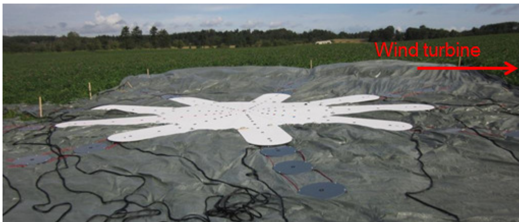
Fig. 3 – The ground array seen from the side, with the right hand side pointing towards the wind turbine.
