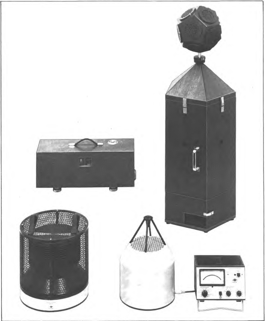
Fig.5.2. Sources of noise: Upper left, Tapping Machine Type 3204; upper right, Isotropic Sound Source Type 4241; Lower left, Reference Sound Source Type 4204; Lower right, Sound Power Source Type 4205
