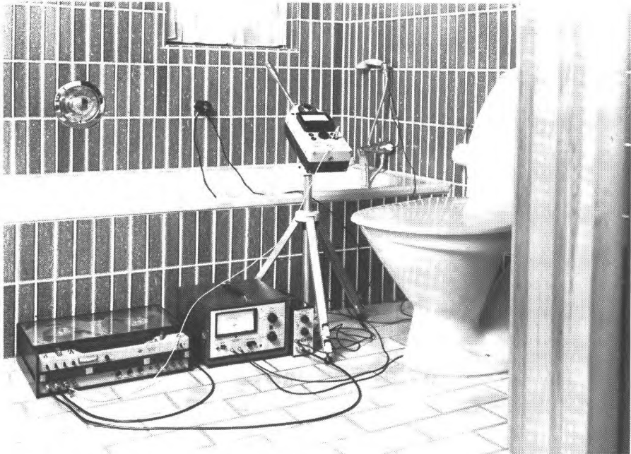
Fig.6.29. Measurement of sound and vibration due to running water
