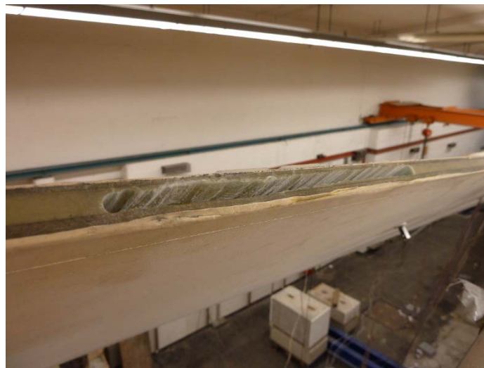
Figure 2: The artificial trailing edge damage introduced in the 34m blade
