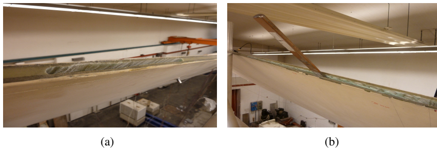
Figure 3 : Debonding introduced in the trailing edge of an SSP 34 m blade. (a) Original drilled debonding. (b) Extended debonding.
