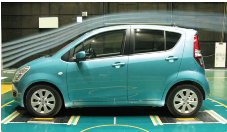
The aerodynamic properties of a Suzuki SPLASH are clearly demonstrated in the wind tunnel
