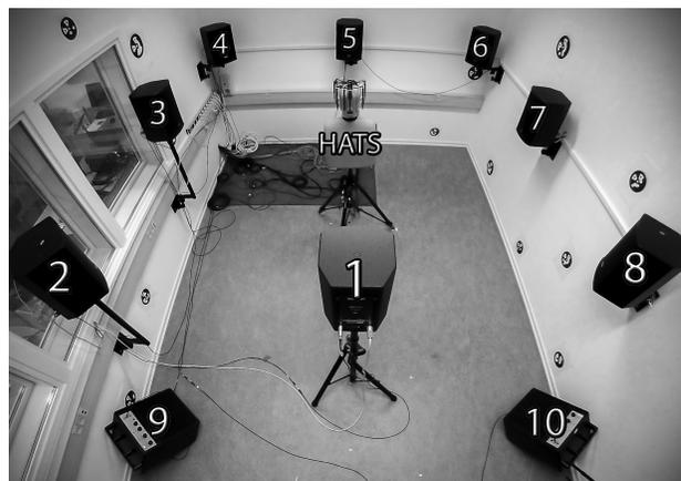
**Figure 3:** Photograph of the reproduction room, the loudspeaker array (1-8), the reference sound sources (9,10), and the HATS with the custom microphone array.
