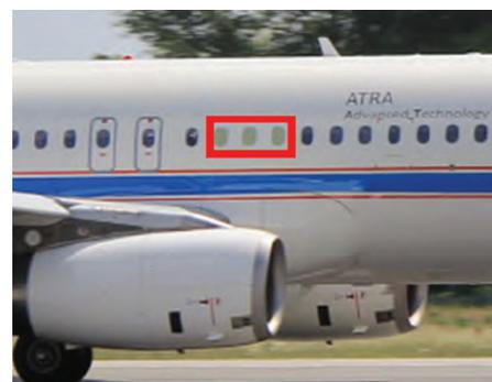
Three false windows held the pressure sensors in the airflow, recessed by 0.3 mm
