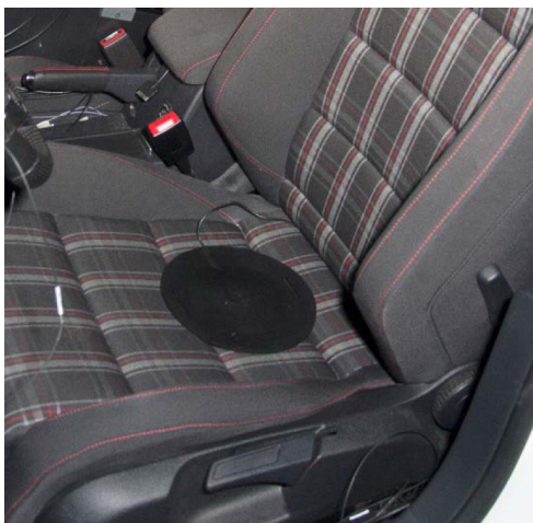
Figure 1. Typical Seat Pad Accelerometer positioning on base of a seat
