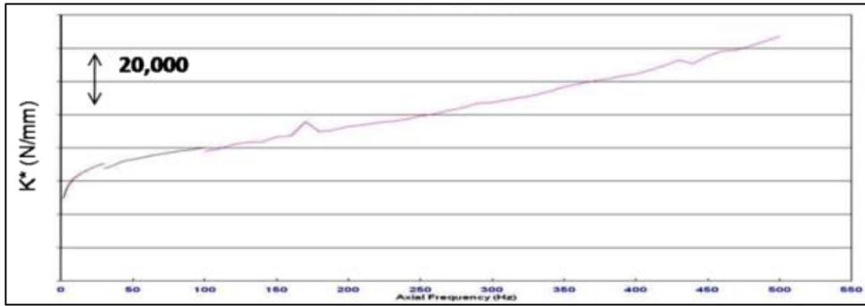
Figure 8: Dynamic stiffness curve for front cab mount
