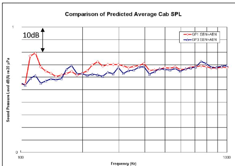
Figure 14. Predicted interior noise spectra for current production (red) and new design machine(blue)
