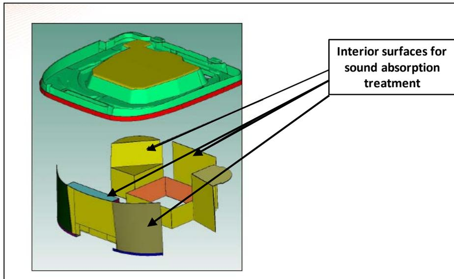
Figure 15: Interior surfaces where sound absorption treatment was simulated.
