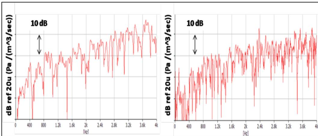
Figure 5: Source-receiver TF, left, local TF (LTF), right, measured using a VVS at the source location.
