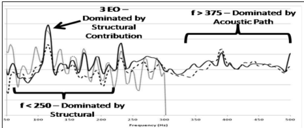
Figure 9. Measured noise spectrum (bold) and estimated structureborne (light gray solid) and airborne contribution (dashed)
