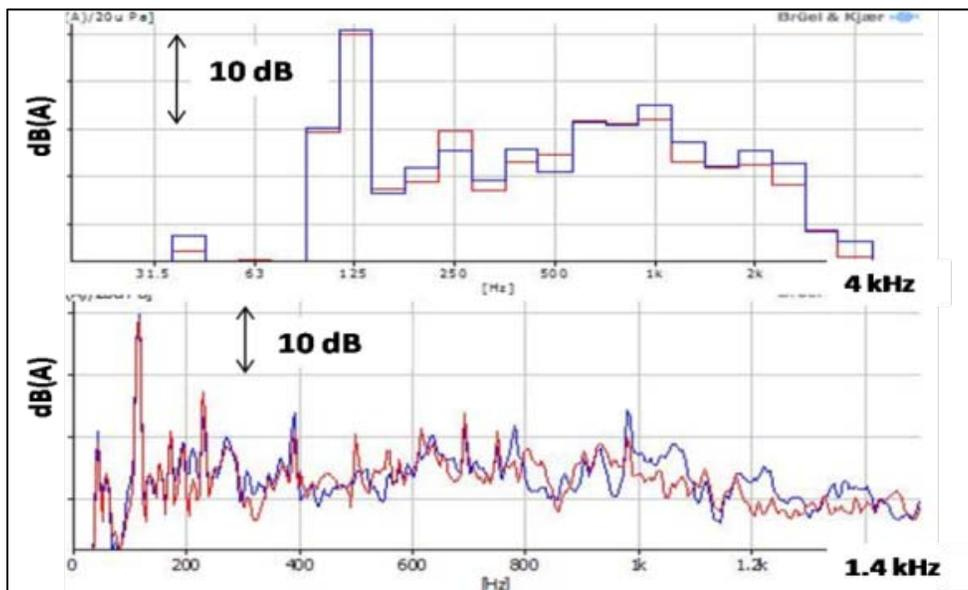
Figure 3. Baseline frequency spectra at driver’s SPL
