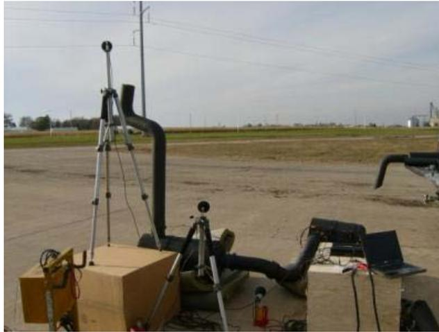
Figure 13: Insertion Loss test set-up
