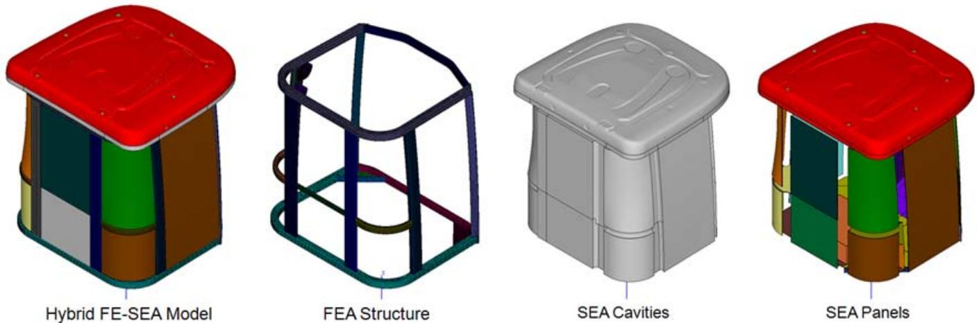
Figure 10. Hybrid FE-SEA model of crop sprayer cab
