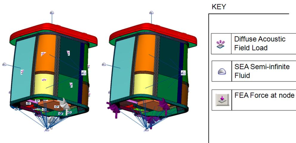
Figure 11: Hybrid SEA/FE model of the cab with the load definitions.
