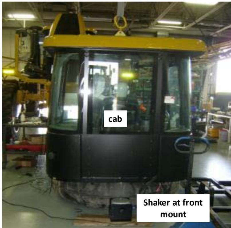
Figure 6: Test set-up using a shaker input to measure the cab transfer functions (P/F).
