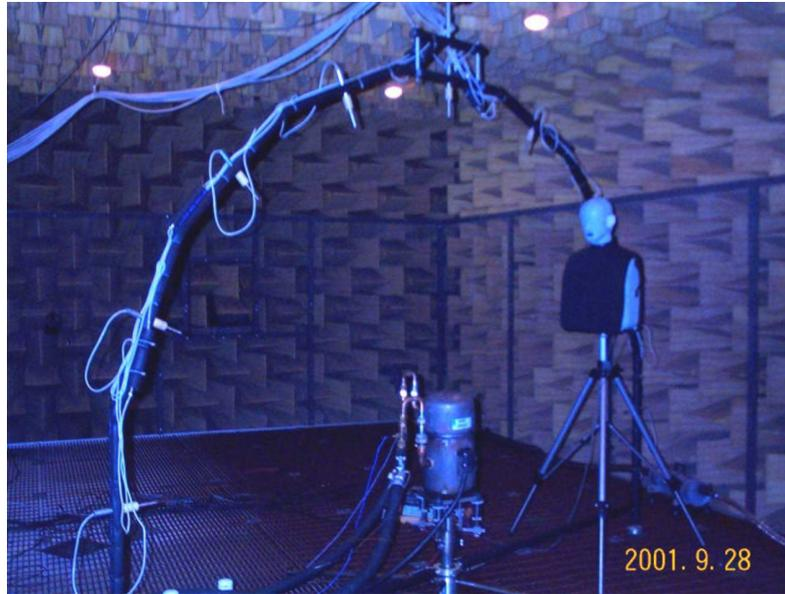
Figure 1: Sound Power Test of compressor in the anechoic room at Tecumseh Products Research Lab
