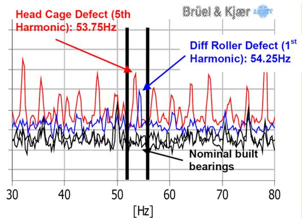
**Figure 6. Separation issue regarding differential rolling defect and head cage defect.**
