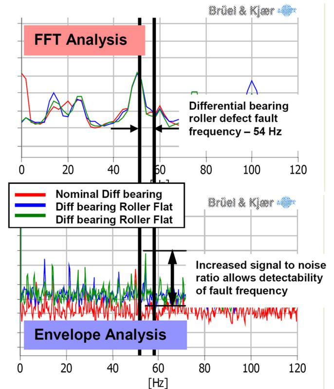
Figure 3. Difference of signal to noise ratio when locating differential bearing roller defect fault frequency (54 Hz) between FFT analysis and envelope analysis.
