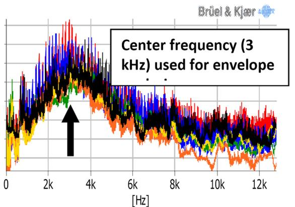
Figure 2. FFT of assemblies with mis-built bearings to determine structural resonance.
