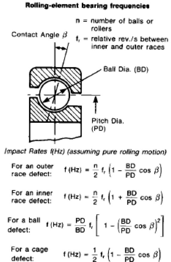
**Figure 1. Formulas for calculating bearing fault frequencies**
