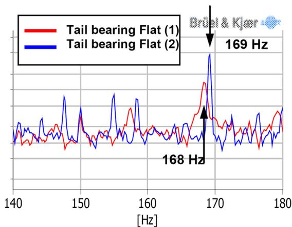
**Figure 4. Slipping effects show that both curves with the same (tail bearing) roller fault frequency can produce slightly different fault frequencies.**
