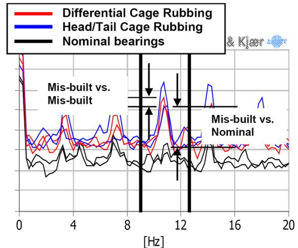
**Figure 5. Separation difference of mis-built bearings and nominally built bearings and also separation of different mis-built bearings.**
